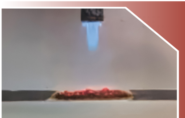
Extended Flame Exposure ( 250°C )
